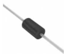
1.5KE6.8CA-E3/51 Vishay Semiconductor Diodes Division TVS DIODE 5.8VWM 10.5VC AXIAL
