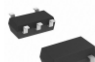
S-80834CLMC-B6TT2G SII Semiconductor Corporation IC VOLT DETECTOR 3.4V SOT23-5
