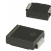
5KASMC24AHM3/57 Vishay Semiconductor Diodes Division TVS DIODE 24VWM 38.9VC DO214AB
