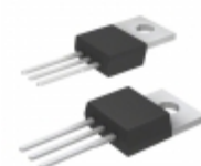
IXTP70N075T2 IXYS MOSFET N-CH 75V 70A TO-220
