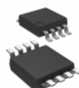
MCP4532T-503E/MS Microchip Technology IC POT DGTL 50K SGL 8-MSOP
