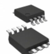
MCP4541-103E/MS Microchip Technology IC DGTL POT 10K 129TAPS 8-MSOP
