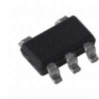
MIC5247-1.55BM5-TR Microchip Technology IC REG LDO 1.55V 0.15A SOT23-5
