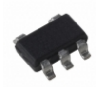
MIC5246-3.3BM5-TR Microchip Technology IC REG LDO 3.3V 0.15A SOT23-5
