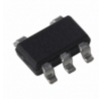
MIC5247-1.5BM5-TR Microchip Technology IC REG LDO 1.5V 0.15A SOT23-5
