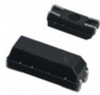
MC-405 32.0000K-R3: PURE SN EPSON CRYSTAL 32.00 KHZ 15.0PF SMD
