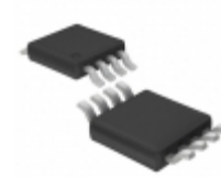
LTC1860LCMS8#TRPBF ADI (Analog Devices, Inc.) IC ADC 12-BIT 1CH 150KSPS 8-MSOP
