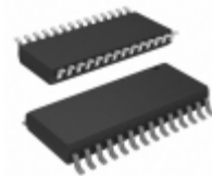
PIC16C642T-20E/SO Microchip Technology IC MCU 8BIT 7KB OTP 28SOIC
