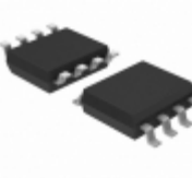
MC908QT2AMDWE NXP Semiconductors / Freescale IC MCU 8BIT 1.5KB FLASH 8SOIC
