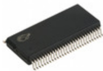
CY7C68001-56PVXC Cypress Semiconductor Corp IC USB INTERFACE SX2 56-SSOP
