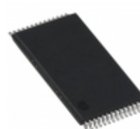
AS7C3256A-20TCN Alliance Memory, Inc. IC SRAM 256KBIT 20NS 28TSOP
