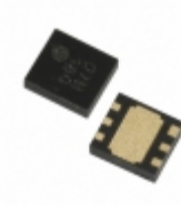
XC6122D719ER-G Torex Semiconductor Ltd IC WATCHDOG TIMER 6-USP
