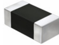
JMK325F476ZN-T Taiyo Yuden CAP CER 47UF 6.3V Y5V 1210
