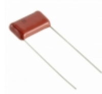
ECQ-E6563JFB Panasonic Electronic Components CAP FILM 0.056UF 5% 630VDC RAD
