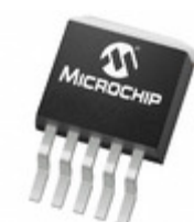
MCP1825-2502E/ET Microchip Technology IC REG LDO 2.5V 0.5A DDPACK
