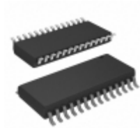
PIC16C63-20/SO Microchip Technology IC MCU 8BIT 7KB OTP 28SOIC
