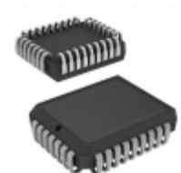
AT49BV002T-12JI Microchip Technology IC FLASH 2MBIT 120NS 32PLCC
