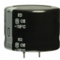
EET-ED2W151EA Panasonic Electronic Components CAP ALUM 150UF 20% 450V SNAP
