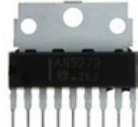
AN5279 Panasonic Electronic Components IC AUDIO AMP 5W SIL-9 W/FIN
