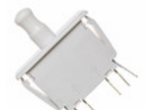
DS2F5CQ3 C&K SWITCH SNAP ACT DPDT 100MA 125V
