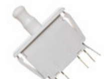
DS2F5CQ1 C&K SWITCH SNAP ACT DPDT 100MA 125V
