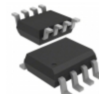
AD8092AR ADI (Analog Devices, Inc.) IC OPAMP VFB 110MHZ RRO 8SOIC
