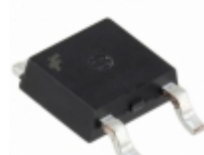
KA78RM33RTM Fairchild/ON Semiconductor IC REG LDO 3.3V 0.5A TO252-3
