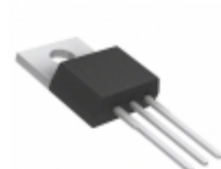
KA78RM33TU Fairchild/ON Semiconductor IC REG LDO 3.3V 0.5A TO220-3
