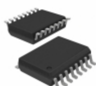
MX7533KCWE+ Maxim Integrated IC DAC 10BIT MULT 16-SOIC
