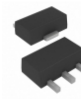
MCP1804T-3002I/MB Microchip Technology IC REG LDO 3V 0.15A SOT89-3
