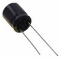
EEU-FC1E681B Panasonic Electronic Components CAP ALUM 680UF 20% 25V RADIAL
