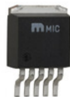
MIC29201-4.8BU Microchip Technology IC REG LDO 4.85V 0.4A TO263-5
