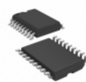
PIC16C716T-04E/SO Microchip Technology IC MCU 8BIT 3.5KB OTP 18SOIC
