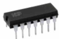
74HC73N,652 NXP USA Inc. IC JK TYPE NEG TRG DUAL 14DIP
