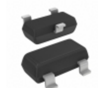
BC860BW,115 Nexperia USA Inc. TRANS PNP 45V 0.1A SOT323
