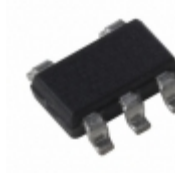
MIC5203-3.8YM5-TR Microchip Technology IC REG LDO 3.8V 80MA SOT23-5
