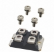
IXFN140N30P IXYS MOSFET N-CH 300V 110A SOT-227B
