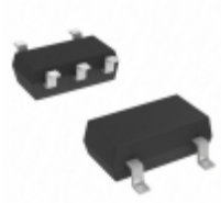
MIC5213-5.0YC5-TR Microchip Technology IC REG LDO 5V 80MA SC70-5
