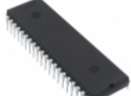
AT87F51RC-24PC Microchip Technology IC MCU 8BIT 32KB FLASH 40DIP
