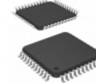
AT87F52-24AC Microchip Technology IC MCU 8BIT 8KB FLASH 44TQFP
