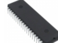
AT87F51RC-24PI Microchip Technology IC MCU 8BIT 32KB FLASH 40DIP
