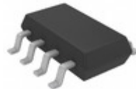
LTC2362CTS8#TRMPBF ADI (Analog Devices, Inc.) IC ADC 12BIT 500KSPS TSOT23-6
