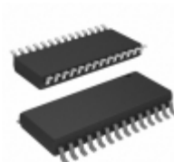
PIC16F1782T-I/SO Microchip Technology IC MCU 8BIT 3.5KB FLASH 28SOIC
