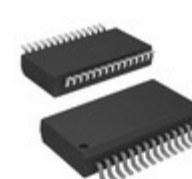
PIC16F1782T-I/SS Microchip Technology IC MCU 8BIT 3.5KB FLASH 28SSOP
