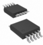
MCP48FVB12T-E/UN Microchip Technology IC DAC SPI 10BIT 2CH NV 10MSOP
