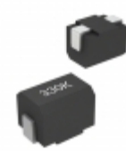
CM453232-471KL Bourns Inc. FIXED IND 470UH 62MA 26 OHM SMD
