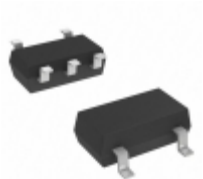
S-8353D50MC-IVJT2U SII Semiconductor Corporation IC REG BOOST 5V 0.3A SOT23-5
