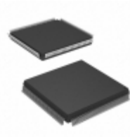
AT40K05-2CQI Microchip Technology IC FPGA 5K GATES 160QFP
