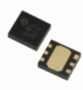
XC6121A741ER-G Torex Semiconductor Ltd IC WATCHDOG TIMER 6-USP
