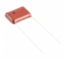
ECQ-E2564RKF Panasonic Electronic Components CAP FILM 0.56UF 10% 250VDC RAD
