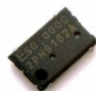
SG-8002JF 46.1000M-PCML3 ROHS Epson OSC XO 46.1MHZ CMOS SMD
