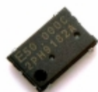
SG-8002JF 46.1000M-PCMB ROHS Epson OSC XO 46.1MHZ CMOS SMD
