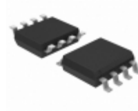
AT24HC02C-SSHM-B Microchip Technology IC EEPROM 2KBIT 1MHZ 8SOIC
