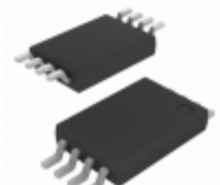
AT24C32A-10TU-1.8 Microchip Technology IC EEPROM 32KBIT 400KHZ 8TSSOP
