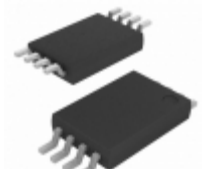
AT24C32A-10TU-2.7 Microchip Technology IC EEPROM 32KBIT 400KHZ 8TSSOP
