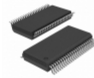
CY14B256LA-SP25XI Cypress Semiconductor Corp IC NVSRAM 256KBIT 25NS 48SSOP
