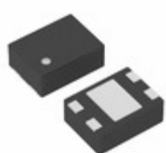
XC6108N22DGR-G Torex Semiconductor Ltd IC SUPERVISOR 2.2V 4-USP
