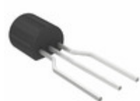
BC239CTA AMI Semiconductor / ON Semiconductor TRANS NPN 25V 0.1A TO-92
