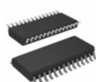
PIC16C642-20I/SO Microchip Technology IC MCU 8BIT 7KB OTP 28SOIC
