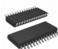
PIC16C642-10I/SO Microchip Technology IC MCU 8BIT 7KB OTP 28SOIC
