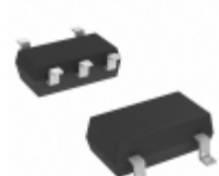
AN80L21RMSTX Panasonic Electronic Components IC REG LDO 2.1V 0.15A MINI5D
